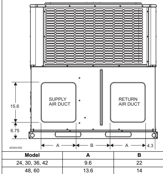
**UNIT TYPICAL DUCT APPLICATIONS**
