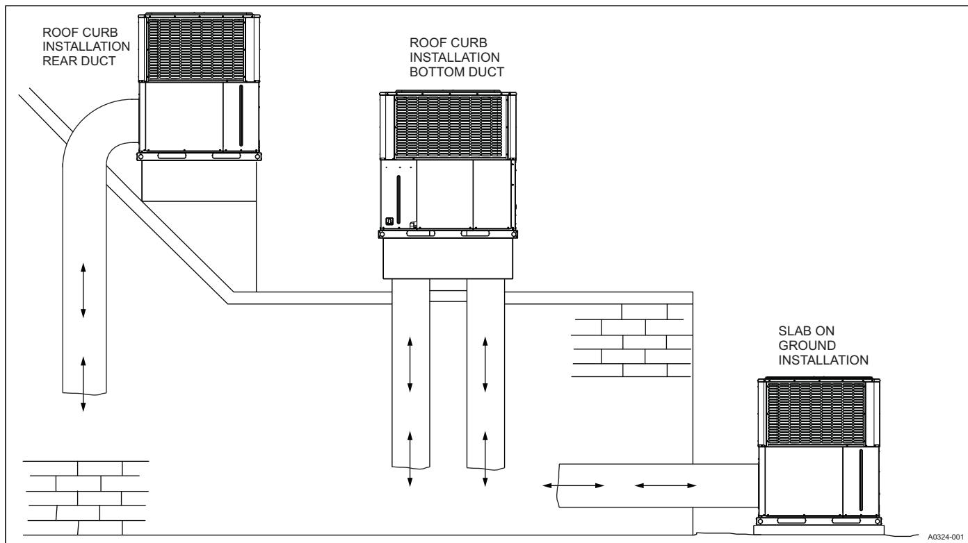
**UNIT TYPICAL SLAB ON GROUND INSTALLATION**
