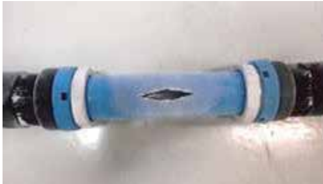
Photo of test at -22°F (-30°C) with NBR seals Pipe bursts at 3527 PSI (243.2 bar) pressure but no failure of the fittings.
