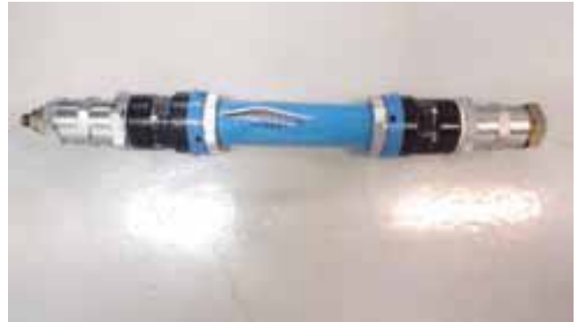
Photo of test at 212°F (+100°C) with NBR seals Pipe bursts at 2942 PSI (202.9 bar) pressure but no failure of the fittings.
