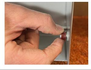
The flat washer limits side-to-side movement of the letter box. It is used if there is no paint on the edge of the pivot pin near the housing.
