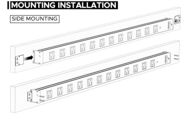
Step 1: Slide one bracket into each end of the power strip
