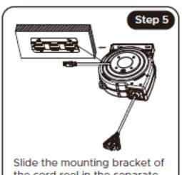
the cord reel in the separate bracket as shown
