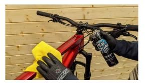
4. To remove any excess adhesive residue, clean with isopropyl alcohol.
