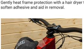
3. Continue to heat and peel until all the frame protection is removed.
