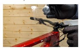
4. Taking one section at a time, spray the frame and protection decal with the soapy water solution.
