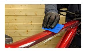
5. Position the decal correctly on the frame using a squeegee to push out water and air bubbles working from the centre outwards.
