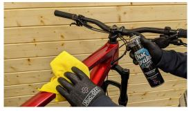
2. Ensure your frame is thoroughly cleaned to remove any dirt and/or grease before starting. Also ensure your hands are clean.
