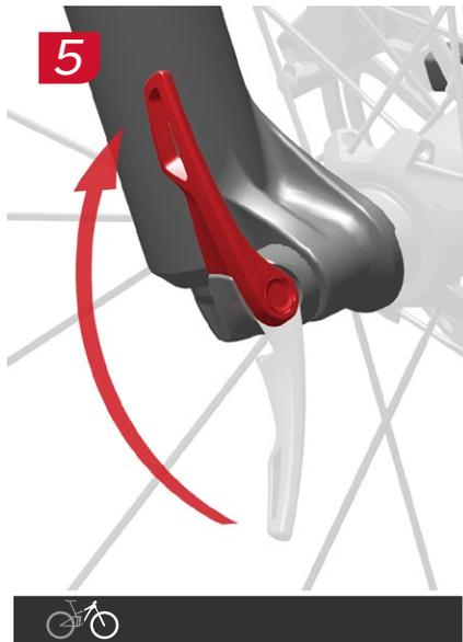
Close the lever and confirm it does not contact the fork or frame. Lever tension is sufficient if the lever leaves an imprint on your hand.
