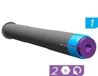
Turn the non-drive side wedge expander counter-clockwise 3 revolutions to loosen the expander.
