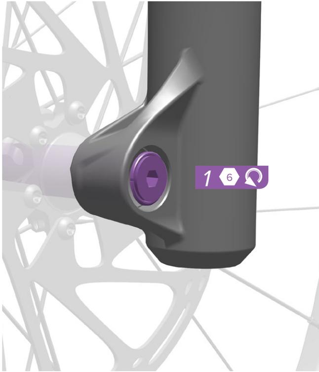
Turn the non-drive side wedge expander counter clockwise 3 revolutions to loosen the expander.
