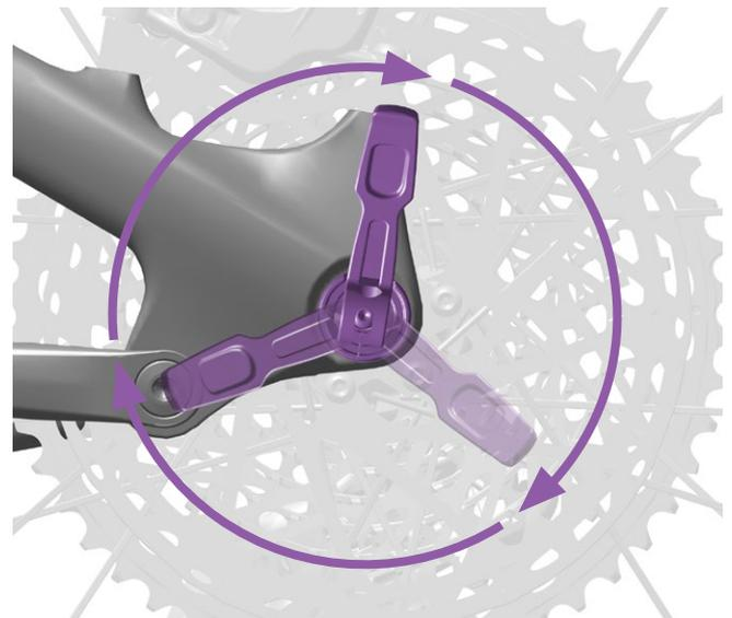
Slide the Maxle™ through the drop out and hub until it contacts the threads of the opposite side drop out. To thread the Maxle into the drop out, rotate the lever clockwise until it stops.
