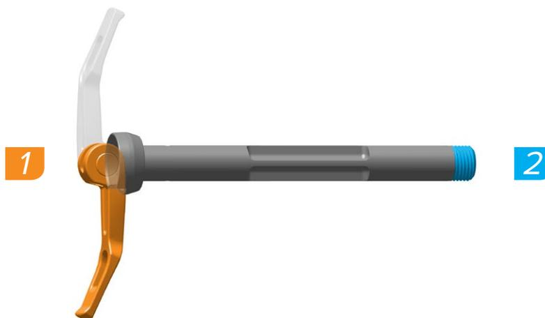
Open the Maxle lever. Ensure the lever rests in the notch on the axle flange.
