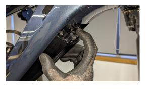
6. Push down the silver clip to fully release the battery.
