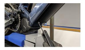
1. Using a 4mm allen key, loosen the bottom 2 bolts of the battery door around 1 full turn (no need to fully remove these bolts).
