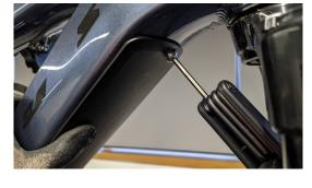
Loosen and fully remove the top battery door holt
