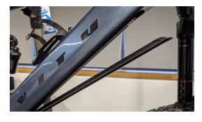
3. Slide the battery door upwards and remove.
