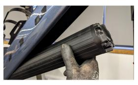
7. The battery can now be removed from the frame.
