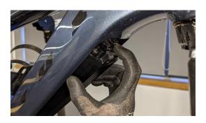
5. The battery should drop down and stop in the position shown.
