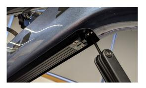
4. Using the 4mm allen key, gently turn the silver battery release bolt **CLOCKWISE** about ¼ turn.
