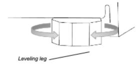
Turning both front legs the same amount to the left will tilt the kegerator to the rear. This adjustment makes it easier for the door to close.
