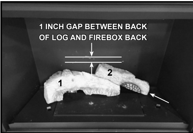
Figure 5. Install Right Rear Base Log
