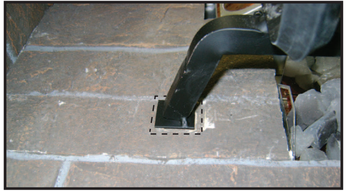
Figure 3. Grate leg placement.
