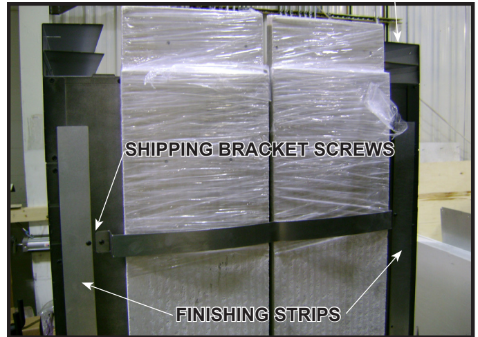
Figure 6.3 Shipping Brackets and Finishing Strip Locations.
