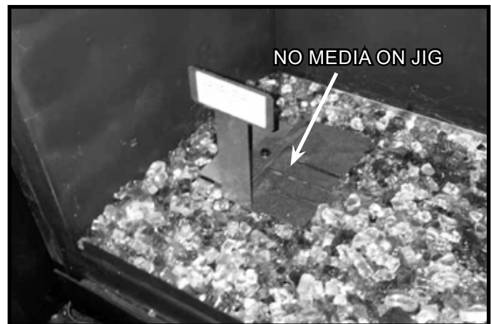
Figure 2. Media Placement Jig in Place
