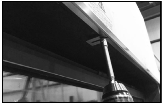
Figure 10.5 Install Trim Ring
