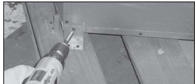
Figure 3.11 Removing Shipping Brackets
