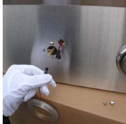
Disconnect the Wire and Change New LEDs
