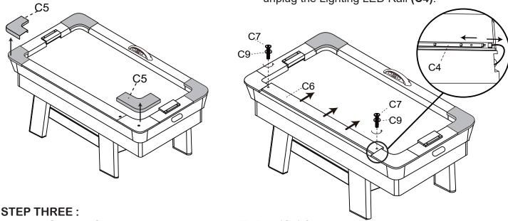
Unscrew Screws (C8), and separate Lighting LED Rail (C4) from each other.
