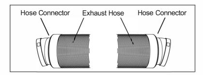
3. Align the tab cut-outs on one of the hose connectors to the tabs on the air exhaust at the rear of the unit and snap in place.
