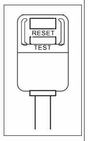
Your portable air conditioner is supplied with a Leakage-Current Detection and Interruption (LCDI) plug. This plug reduces the risk of fire due to arcing faults in the power supply cord. Please follow the instructions below to ensure that LCDI plug works properly.
