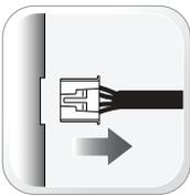
Disconnect the M1 BLACK 8-pin connector and the M4 BLACK 20-pin connector.
