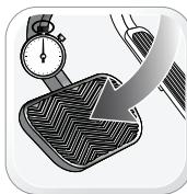
Press and hold the brake pedal.
