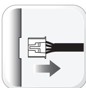
Disconnect all connectors from module except the M1 BLACK 8-pin connector and the M4 BLACK 20-pin connector.
