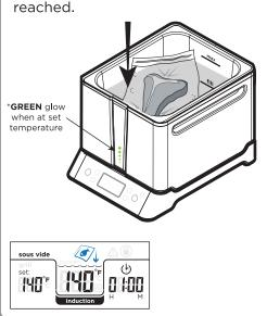
**5.** Optional timer setting: You can press the timer button to set a timer. When the temperature is stable, you can activate the timer by pressing start.
