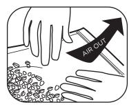
4 Lay the bag flat, placing the indicator circle directly over the arrow on the drip tray.
