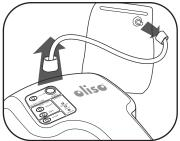
NOTE: Keep the Flexi Tube connected to the Oliso® PRO™ Smart Vacuum Sealer if you want to continue using accessories. You must disconnect the Flexi Tube from the vacuum sealer before using a Vac-Snap® bag.
