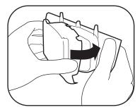
Remove the orange gasket. Do not remove the black rubber ring. Wash each piece with warm soapy water. Dry completely before reassembling.
