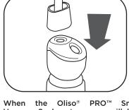
Vacuum Sealer stops you will hear two beeps and see the DONE light illuminate. Twist to disconnect hose.
