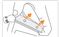
**Gently** loosen cover by lifting directly away from iron. Cable and cover will remain attached to iron.
