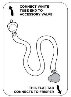
NOTE: Disconnect flexi tube by twisting the flat tabbed end counterclockwise. You must disconnect the flexi tube before using Frisper with vac-snap zipper bags. 1 Connect white tube end to accessory valve.
