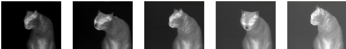
Figure 3-1 Adjust Brightness in White Hot Mode
