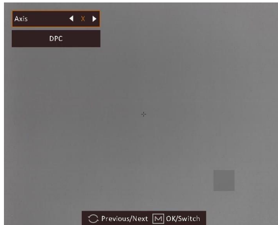
Figure 3-3 Correct Defective Pixel
