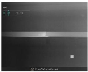
• If the screen OSD blocks the defective pixel, move the cursor to reach the defective pixel, then the device performs mirror display automatically.
