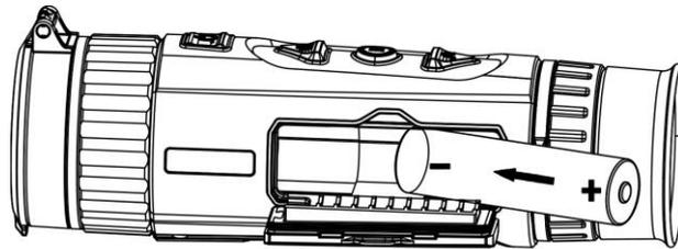
Figure 2-4 Install Battery
