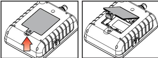
**Step 2:** Place battery in correctly, put the battery cover back on.
