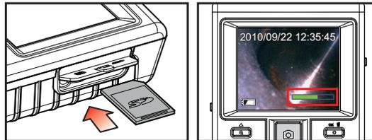
**Step 5:** Hold down the monitor ON/OFF switch until monitor screen display is visible.
