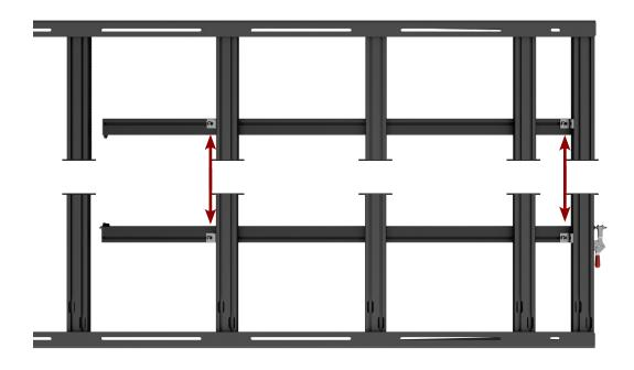
Align the latch plate with the edge of the extrusion when positioning the table. Repeat this on the opposite side.
