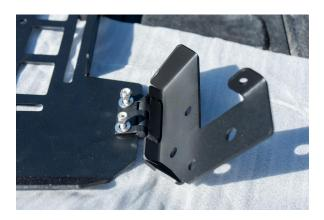
To mount the Rear Door to the Driver Side Mounting Hinge and the Passenger Side Mounting Hinge, you will use (2) ¼ - 20 Nylon Nuts and (2) ¼" Stainless Steel Washers, threading them onto the threaded studs on the Rear Door on each side.
