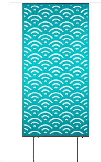
Direct fixed top suspended base
