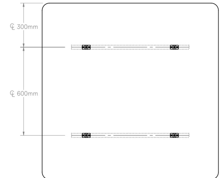
3. Using suitable screws for the wall substrate (not supplied), screw the RAFNEX24 channels to the wall in the relevant locations.
