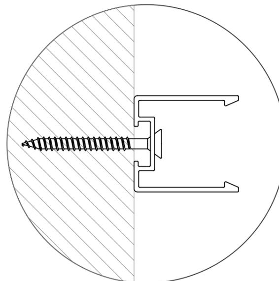
4. Carefully lift the Horizon panel into place and clip the Floating Panel Connectors into the RAFNEX24 channel.
