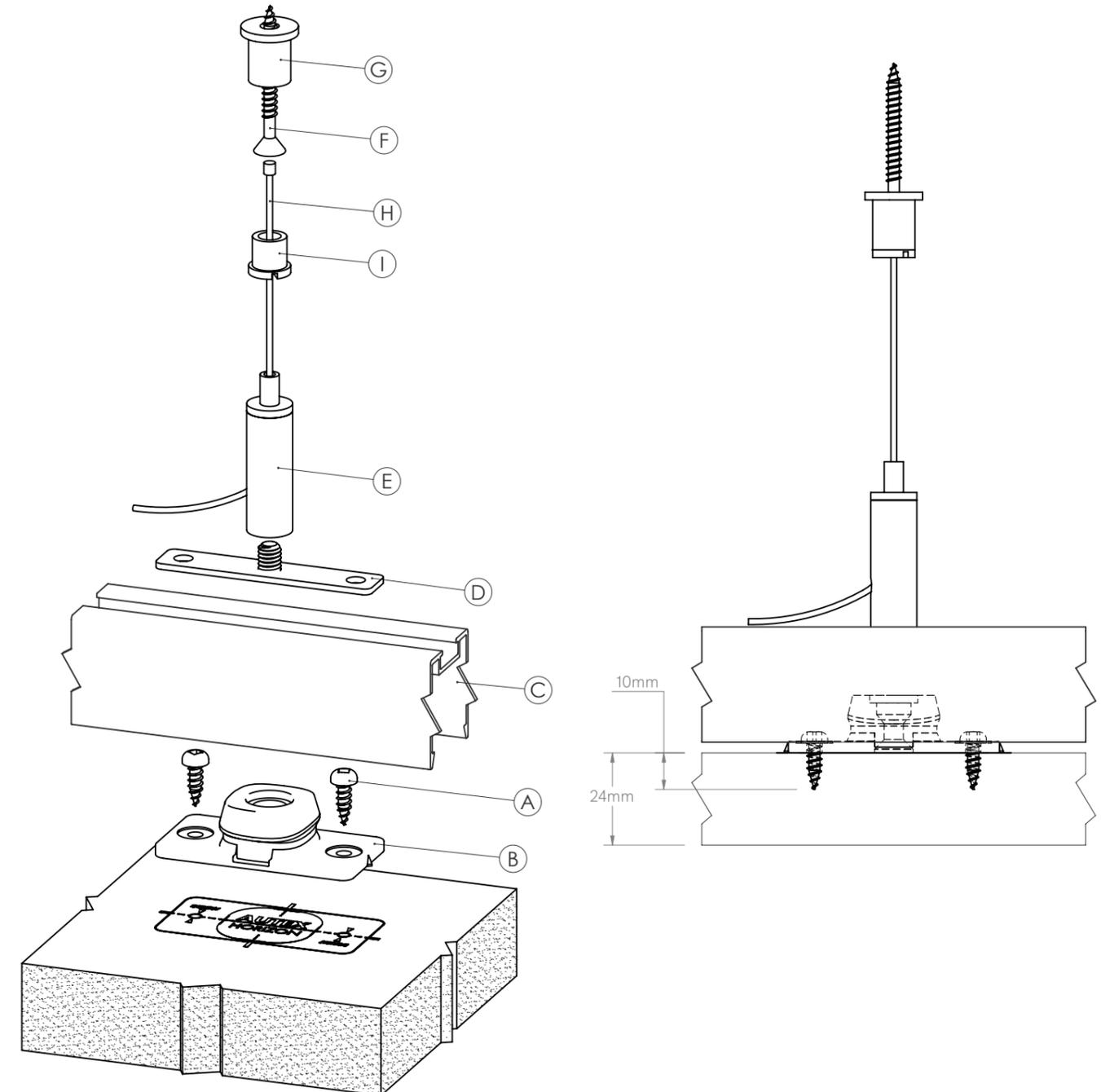
1. Using the supplied 12mm panhead screws (A), attach all the Floating Panel Connectors (B) to the Horizon panel. Use the positions marked on the Horizon panel to correctly position the Floating Panel Connectors.
