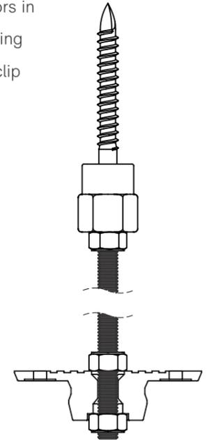
4. Lift the RAFNEX24 channel and clip into place, aligning the Floating Panel Connectors with the length of the extrusion.
