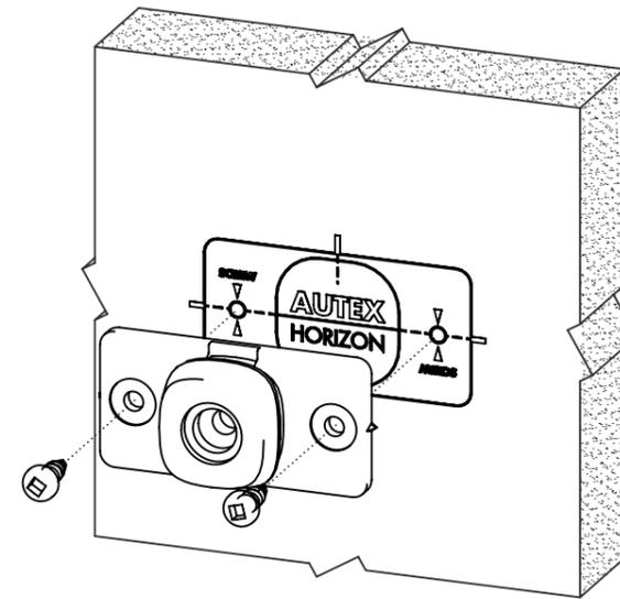
2. Measure the vertical distance from the centre of the Floating Panel Connectors to the top of the panel and make note of this when screwing the RAFNEX24 channel to the wall.
