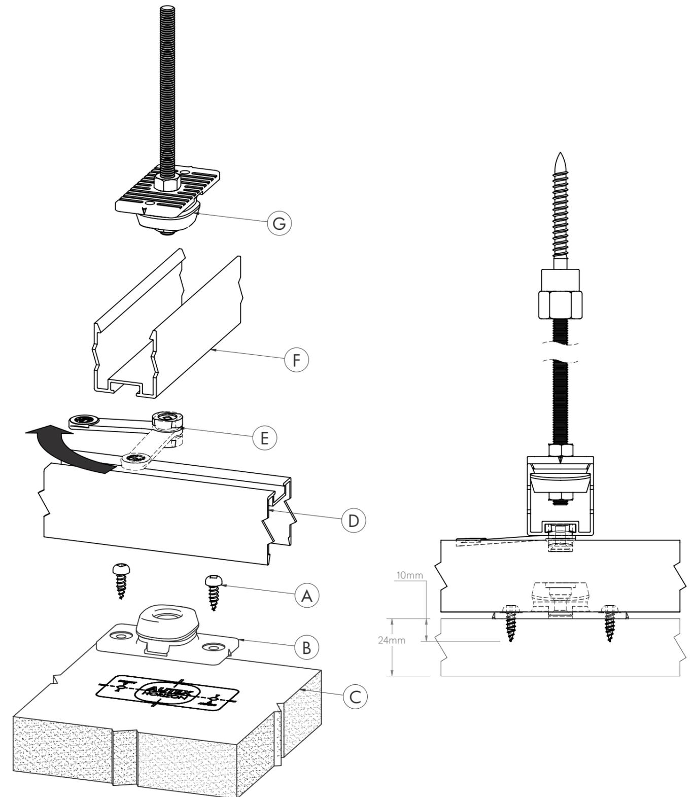
1. The Floating Panel Connectors in the RAFFPC set are designed to fit a M5 Countersunk screw.
