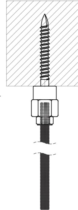
3. Affix the Floating Panel Connectors in place on the threaded rods by using nylok nuts above and below the clip to set its height.
