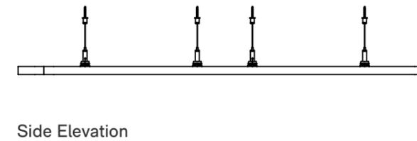
**Note:** Suspension Method 2 could also be used to hang these panels, reducing the number of hangers required.
