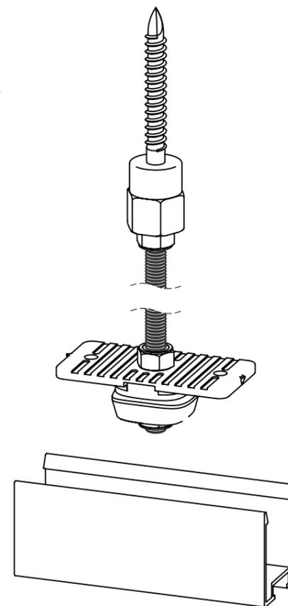
5. Should further adjustment to the heights be required, you can remove the channel from the Floating Panel Connectors.
