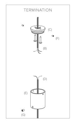
A Before starting, determine which fasteners will be best suited to secure the fitting, based on the material of the ceiling substrate.
