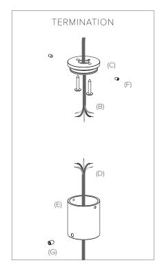
⚠ Before starting, determine which fasteners will be best suited to secure the fitting, based on the material of the ceiling substrate.
