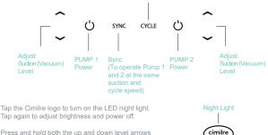
Press and hold both the up and down level arrows of either side for 3 seconds to mute or unmute sound.
