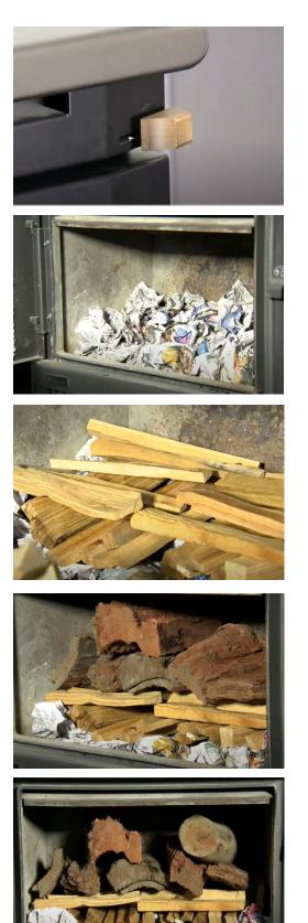
Shift the air slide control knob to the RIGHT hand side, this allows more oxygen in the firebox and will ensure the fire can start easily.
