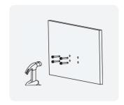
Knock the wall insert bolts into the wall and&lossen the srews nuts.
