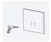
Mark the hole location where you want to mount.Drill 4 holes as per the location.
