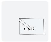
Fix the bracket on the wall with screw nuts.
