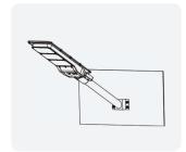
Adjust the angle of the lamp and fix it on the bracket.
