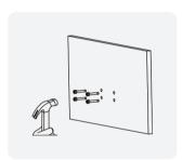
Knock the wall insert bolts into the wall and&lossen the srews
