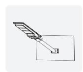
Adjust the angle of the lamp and fix it on the bracket.
