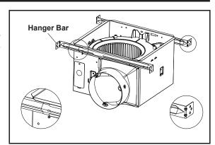
2.Extend the hanger bars to the width of the framing. Position the ventilator with the bottom edge of the hanger bar tabs are flush with the bottom edge of the framing, holding the ventilator in place. Secure hanger bars to framing using one screw on each end of hanger bar. Select a proper hole and secure the hanger bars together using one screw.
