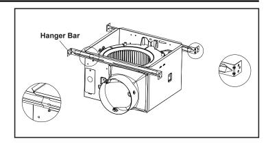
2.Extend the hanger bars to the width of the framing. Position the ventilator with the bottom edge of the hanger bar tabs are flush with the bottom edge of the framing, holding the ventilator in place. Secure hanger bars to framing using one screw on each end of hanger bar. Select a proper hole and secure the hanger bars together using one screw.
