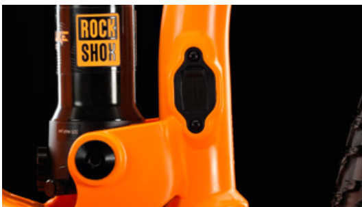
BATTERY CHARGER: Battery charger port is located on the seat tube.
