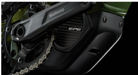
DRIVE UNIT: Special cover protect the engine from impacts.
