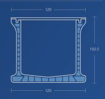
Water Flow 825 L/M Open End Discharge 0.5 Fall to Cesspit
