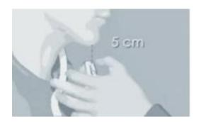
5. Press and hold the two volume keys (+/-) simultaneously for at least five seconds. When a beep is heard through your hearing aids the RC-DEX is matched.
