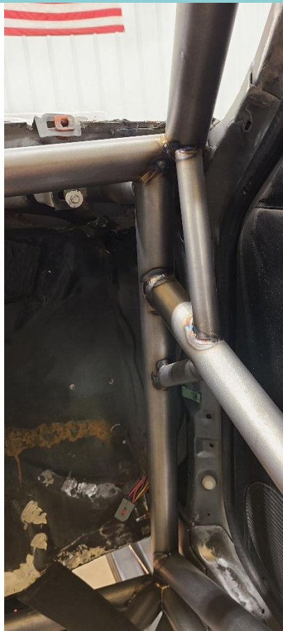
Dash bar and gusset placement
