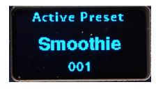
When using this mode, the OLED screen displays the name of the active Preset and number. Presets are arranged as a list and sorted based on the preset number.
