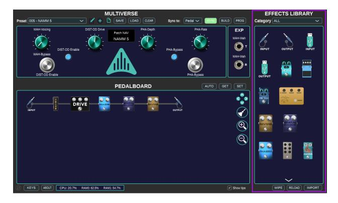
By default, the *Effect Library* contains four components. Stereo *TRS Input* and *TRS Output* for the ¼" TRS connections on the Multiverse pedal, as well as stereo *USB Input* and *USB Output* for acting as a USB audio device. *Note: USB audio is currently an experimental feature*.
