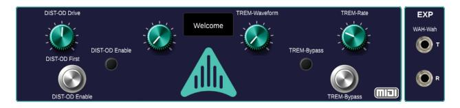
This section of the application provides a virtual representation of the hardware pedal. The Multiverse pedal provides four rotary encoders, four encoder push-buttons, two stomp switches, and two LEDs, all of which are assignable to control your audio effects.
