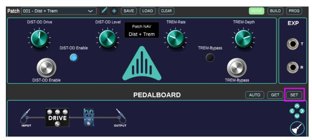
f) When finished, don't forget to click the *Pedalboard* **SET** button to save these settings into the preset.
