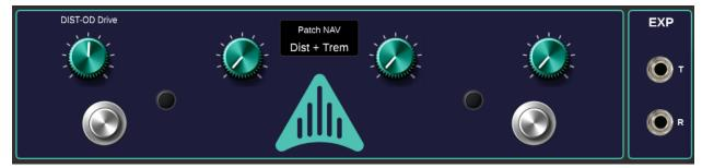
Notice that the name of the effect (DIST) and the control (OD Drive) now appeared above the knob. We have now assigned this knob on the *Multiverse* pedal to control the OD Drive control when this preset is active.
