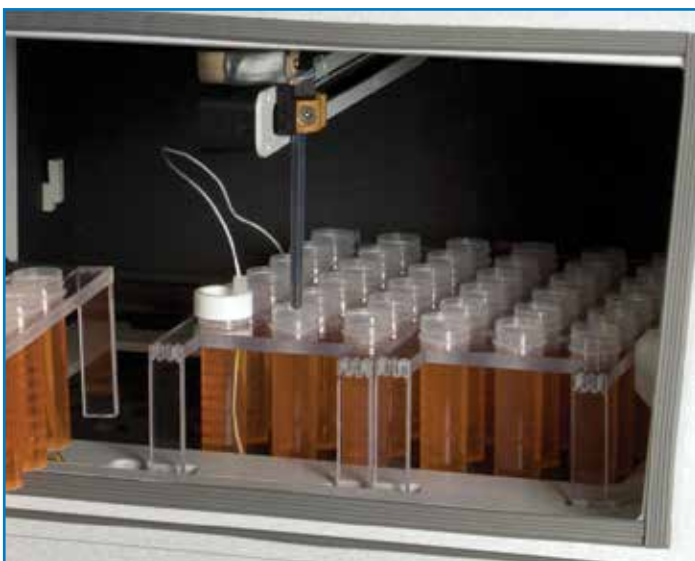
A PTFE thermocouple, placed in a designated reference well continually tracks sample temperature
