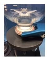
• Rinse the funnel and disk with a small volume of n-Hexane to clean the system and direct to waste.
