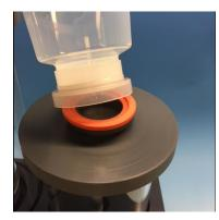
• If using the glass funnel, add the orange gasket and stainless steel support screen to the platform.
