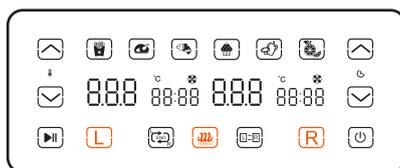
3. Use the TEMP arrows to set the temperature. (Time will end automatically according to the preset temperature).
