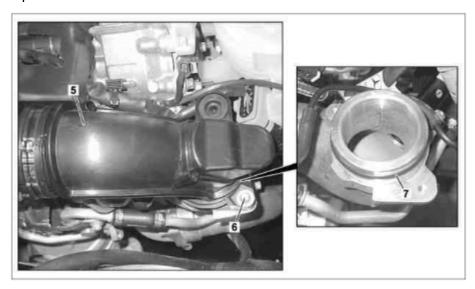
4. Pull up on each airbox to unseat it from the turbocharger. **NOTE:** Each turbocharger has a seal (item 7).
