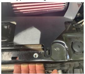
d. GEN 1 Intake systems require mounting adapter, GEN 2 (Nov 2020 and later) do not. If you have a Gen 1, Install the heat shield mounting block to the chassis by placing the M6 bolt through the block and tighten the nut, otherwise clamp heat shield directly to chassis.
