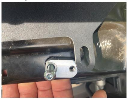
e. Clamp heat shield to the block with the short M6 screw. This may need to be adjusted during the reinstallation of the plastic ram air inlet
